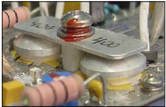
Device clamp to insure good thermal
