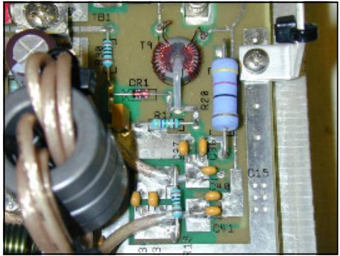
RF balance transformer and alarm
